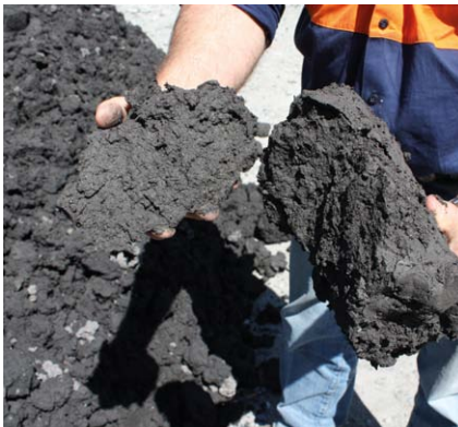
The output from an Alfa Laval decanter centrifuge is sufficiently dry to be stacked.
